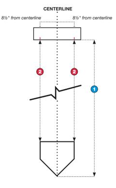
When all of these 4 parameters have been met — elevation, distance, level, and square — make sure to double-check all of the measurements one last time before finally backfilling around the rubber. After compacting around the rubber, do one final check on level, distance, and square to insure the compacting process did not throw the rubber off its mark.
