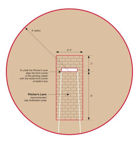
The **Softball Pitching Circle** is a 16' diameter circle. The center is located along an invisible line extending from the apex of home plate through the center of 2nd base. The front, center edge of the pitching rubber is located in the center of the 8' radius pitching circle. The distance of the pitching rubber from the apex of home plate varies from 35' - 50'. Consult the Softball Field Dimensions Diagram earlier in this guide for the appropriate distance for your governing body and league.
